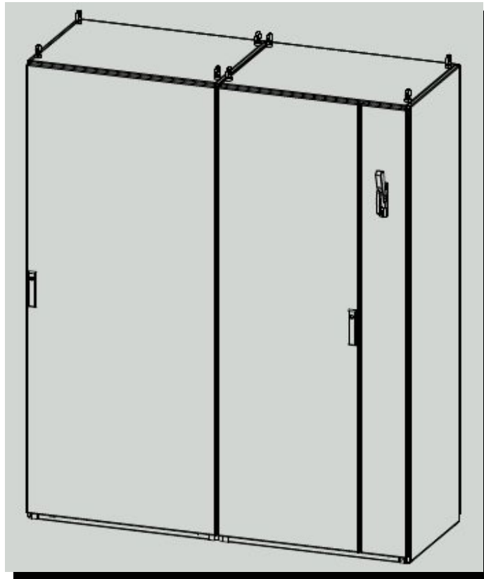
Sample disconnect system with right-mounted master disconnect and slave cabinet mounted to left
